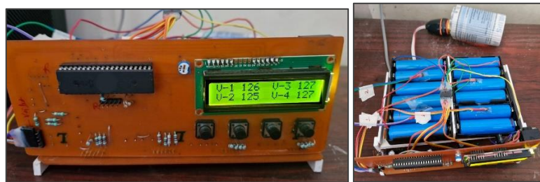
Figure 6: Hardware setup with microcontroller and batteries
