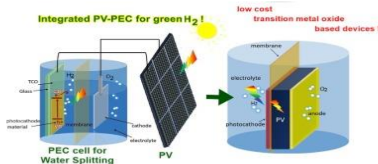
Figure 3. Photovoltaic Electro Catalysis Integration System for Green Hydrogen [33]
