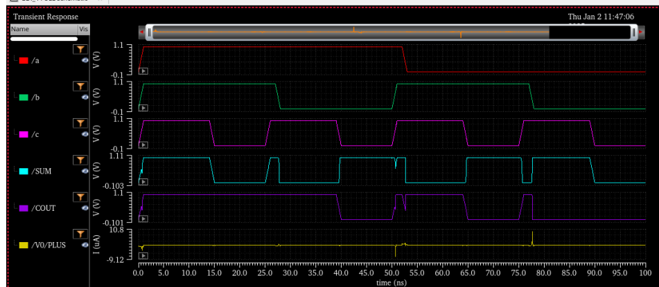
Fig.16: MUX Based Full Adder Input& Output Waveforms
