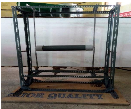
Figure 3.1: Experimental set up (prototype model) of VIVWPGEN with foundation structure.
