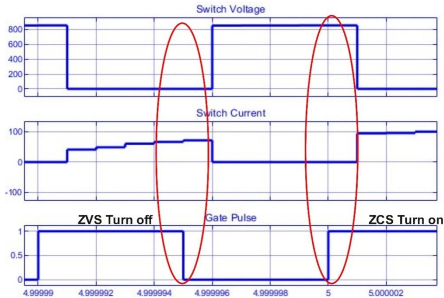
Figure 6: Simulation results showing ZVS and ZCS of switch S1
