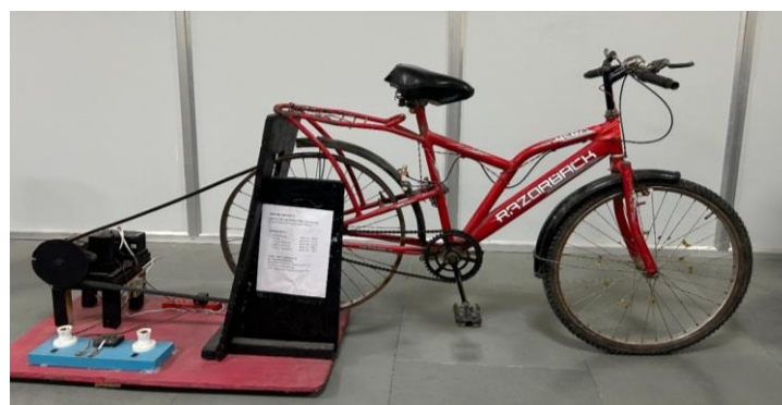
Figure 3. Laboratory Setup of Pedal Powered Generation System
