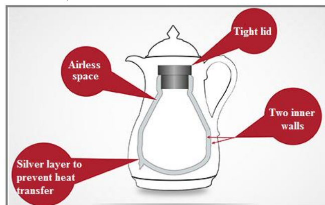
Schematic diagram of the components of a thermos
