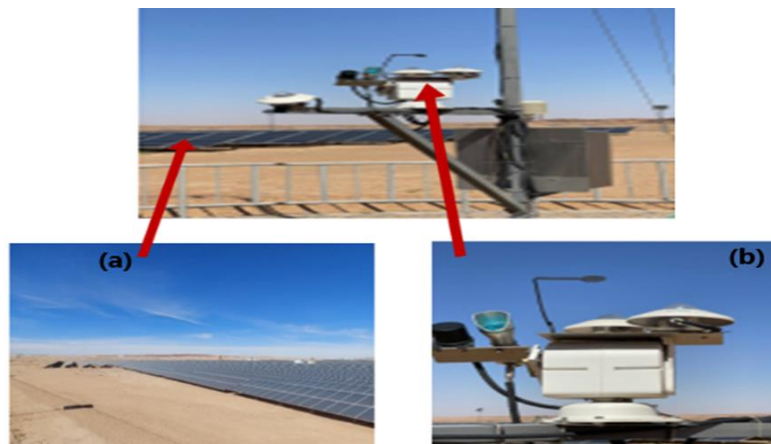
Figure 2. (a) The photovoltaic station under study, (b) the climate data monitoring unit.
