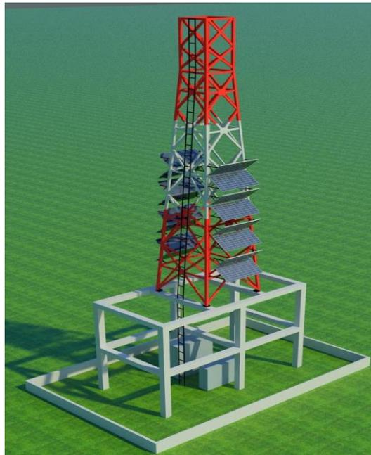
Figure 3: Installing bi-facial panels in the existing 42m communication tower
