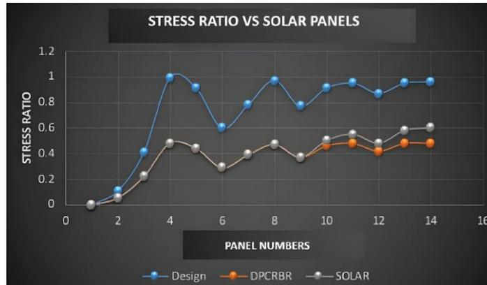
Figure 4: Stress Ratio of 42m Communication Tower with Bi-facial Panels
