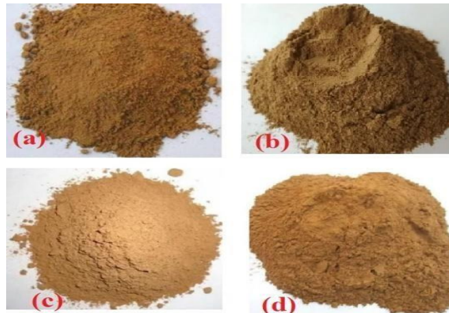
Fig. 4 Photographs of CS powder of sizes (a) 400 \mu\text{m} , (b) 300 \mu\text{m} , (c) 150 \mu\text{m} , and (d) 100 \mu\text{m}
