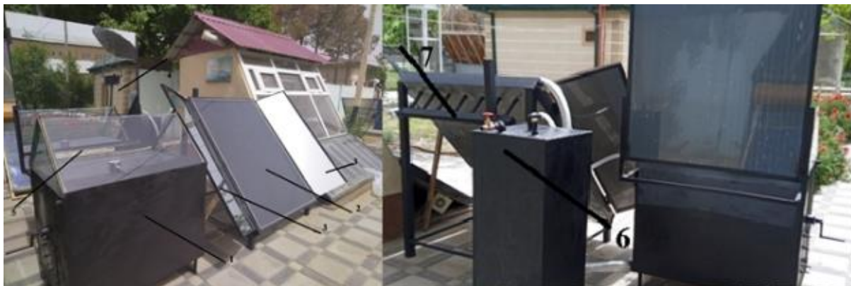
Figure 3. Experimental setup of a heliothermal household waste treatment plant.
