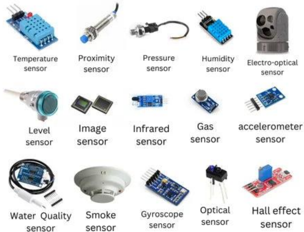
Figure 2: Types of IoT sensors used in heat transfer monitoring
