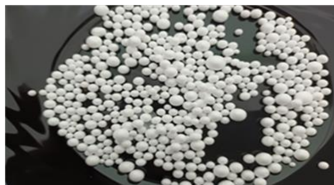
Figure 2. Expanded polystyrene (EPS) beads with different diameter.
