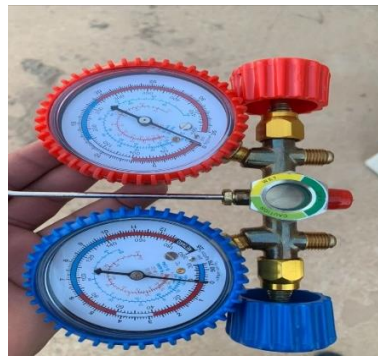
Fig. 5 Measuring instruments including a manifold gauge for refrigerant pressure
