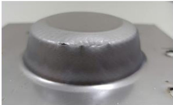
Fig. 10 Model 7. Crack initiation at stage 6 ( \alpha_6 = 74^\circ ): (m) finite element prediction; (n) experimental observation.
