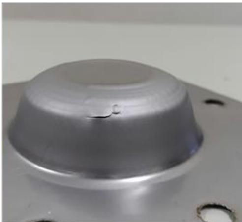
Fig. 11 Model 8. Specimen achieving a forming angle of 84^\circ under the optimal parameter combination: (o) finite element prediction; (p) experimental observation. The sheet was successfully formed to \alpha_8 = 84^\circ without fracture, confirming the consistency between numerical simulation and experimental results.
