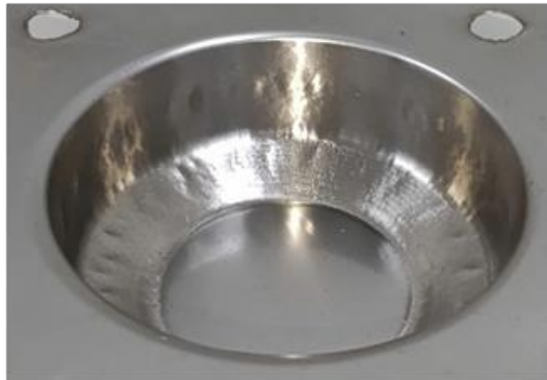
Fig. 11 Model 8. Specimen achieving a forming angle of 84^\circ under the optimal parameter combination: (o) finite element prediction; (p) experimental observation. The sheet was successfully formed to \alpha_8 = 84^\circ without fracture, confirming the consistency between numerical simulation and experimental results.
