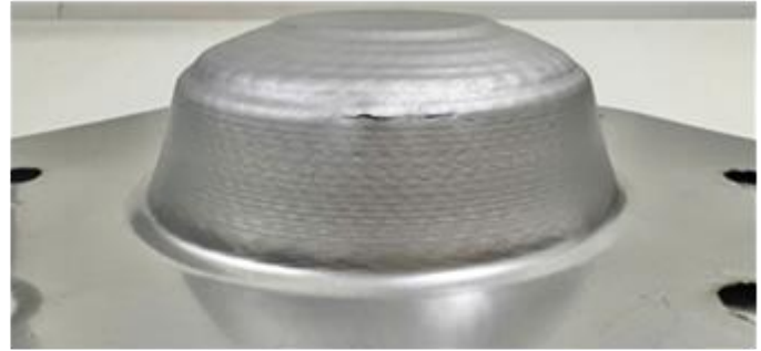
Fig. 4 Model 1. Crack initiation at stage 6 ( \alpha_6 = 72^\circ ): (a) finite element prediction; (b) experimental observation.
