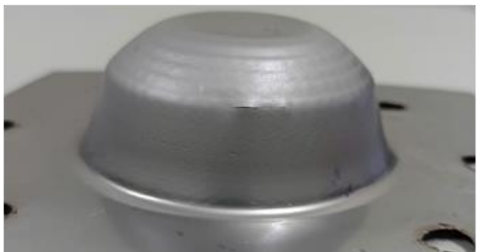
Fig. 6 Model 3. Crack initiation at stage 6 ( \alpha_6 = 72^\circ ): (e) finite element prediction; (f) experimental observation.
