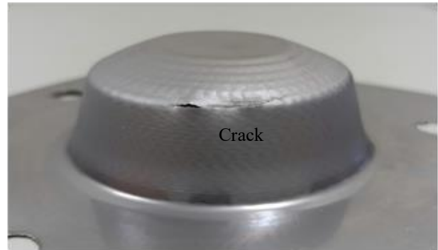
Fig. 7 Model 4. Crack initiation at stage 6 ( \alpha_6 = 74^\circ ): (g) finite element prediction; (h) experimental observation.
