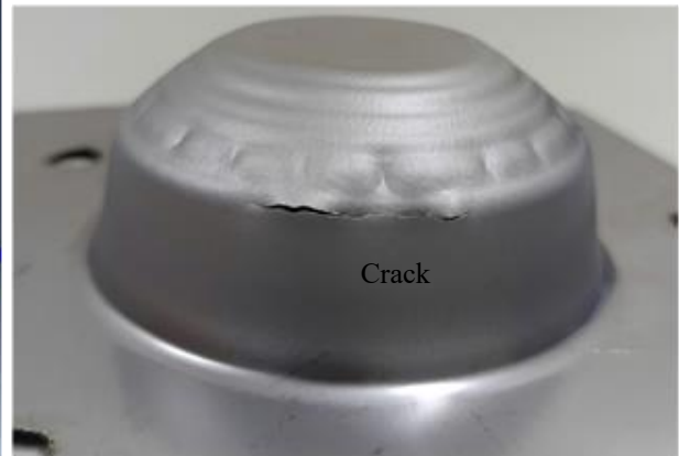
Fig. 8 Model 5. Crack initiation at stage 7 ( \alpha_7 = 79^\circ ): (i) finite element prediction; (j) experimental observation.
