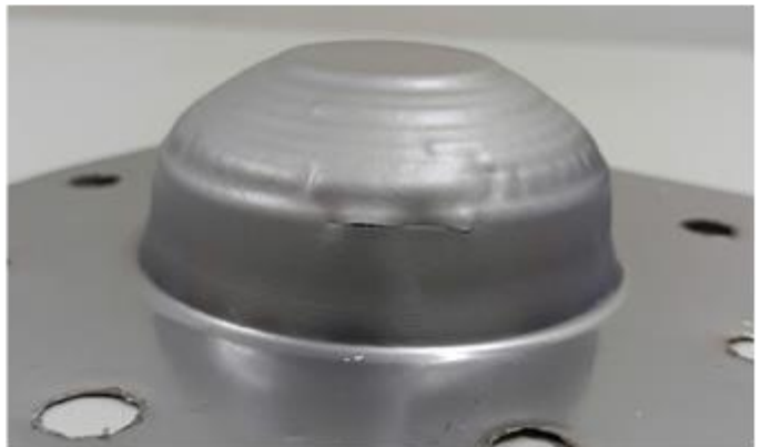
Fig. 5 Model 2. Crack initiation at stage 8 ( \alpha_8 = 82^\circ ): (c) finite element prediction; (d) experimental observation.
