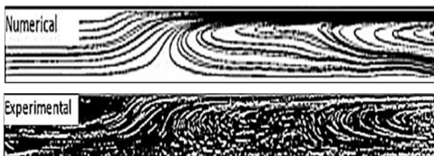
Fig. 2 Validation between experimental and simulation results for Ra^* = 4.5 \times 10^6 .
