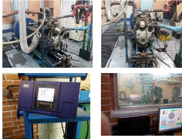
Figure 5. Physical Configuration of the Dual-Fuel Ignition Compression Engine (MT440C Model)
