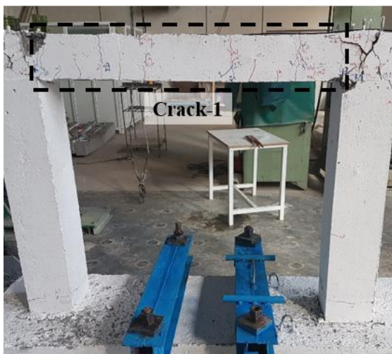
Figure 13. Cracking way of the ConcF-3 after the experiment concrete frame in numerical modeling
