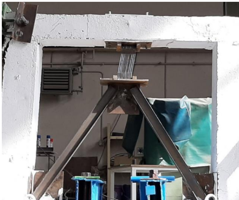
Figure 17. Concrete frame with the yielding ADAS damper of the F-3-ADAS sample
