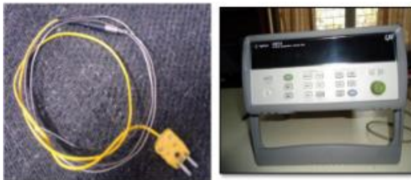
Figure 5: K-type thermocouples for measuring temperature
