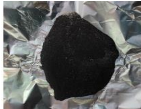
Figure 3: Silicon carbide particles of 40µm
