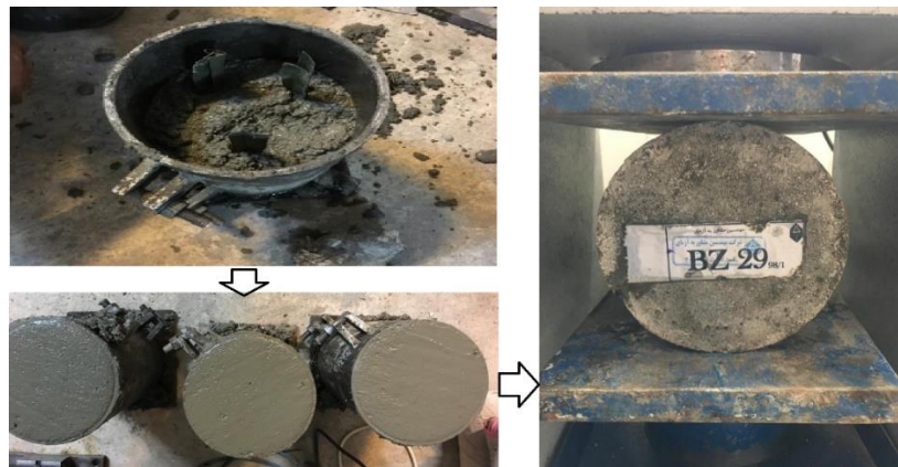
Fig 16: steps of making concrete sample and Brazilian test
