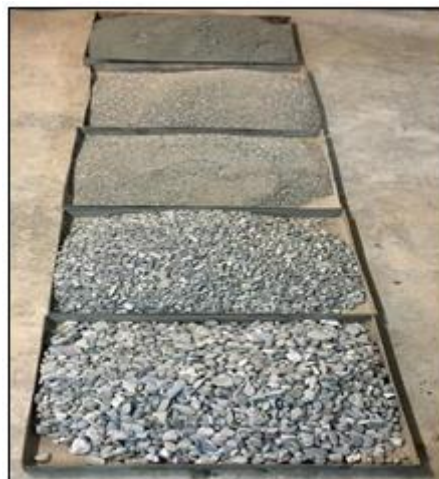
Fig 11: sieved materials in order of size to prepare the mixing plan
