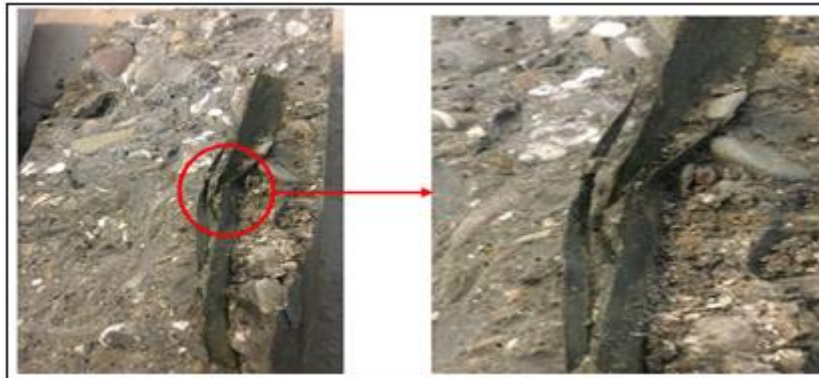
Fig 18: Cylindrical concrete sample after applying pressure and breaking the leaves in the concrete
