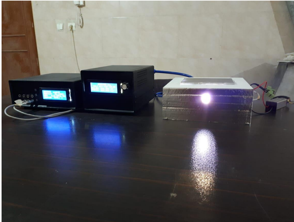
Figure 11. Starting the test for the radiant light spectrum on the surface of concrete to perform the photocatalytic activity of concrete to absorb nitrogen oxide gas around the surface of the sample in the test device.
