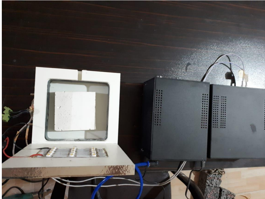
Figure 9. Placing the concrete sample in the device to carry out the photocatalytic activity of concrete to absorb nitrogen oxide gas around the surface of the sample in the test device.
