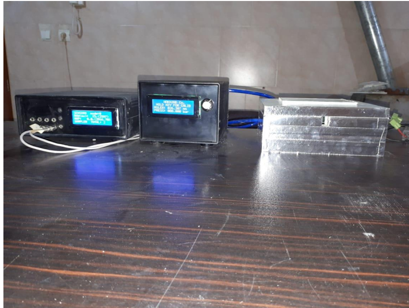
Figure 5. Device for determining the amount of reduction of nitrogen oxide adjacent to the samples in the tested designs
