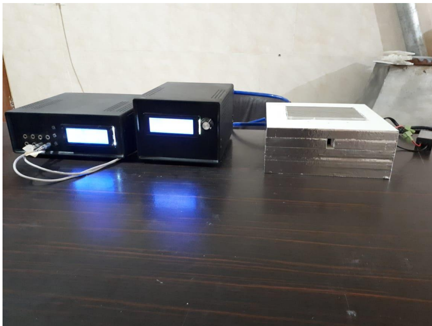
Figure 6. Device for determining the amount of reduction of nitrogen oxide adjacent to the samples in the tested designs
