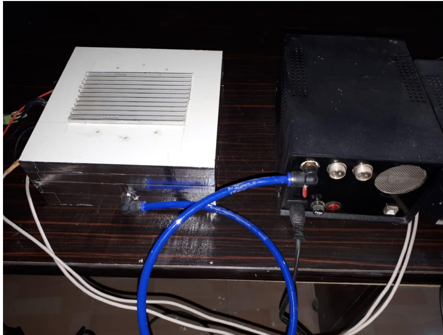
Figure 7. The input of nitrogen oxide gas from the tank to the surface of the sample in the test device to determine the reduction of nitrogen oxide adjacent to the samples in the tested designs.
